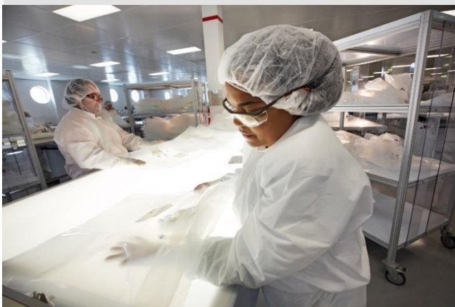
Visual inspection of SUS process equipment for visible particles >100\mu\text{m}
