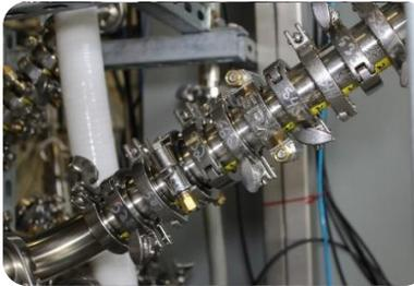
BPI designed a life cycle performance test for the client's prototype gasket, comparing it to other commercially-available gaskets across three sizes with respect to multiple performance criteria. The gaskets were successfully exposed to Steam-In-Place (SIP) cycles.
